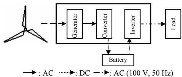
Fig.1. Basic structure of small wind turbine.
