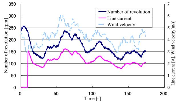
Fig. 10. Number of revolution and line current (Discharge equipment, average wind velocity: 4.2[m/s]).
