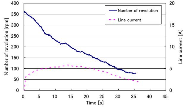
Fig. 9. Number of revolution and line current (1R30A×3, average wind velocity: 5[m/s]).
