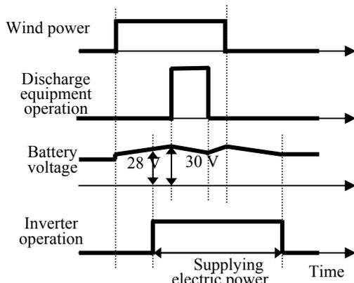
Fig.5. Operation model of control system.
