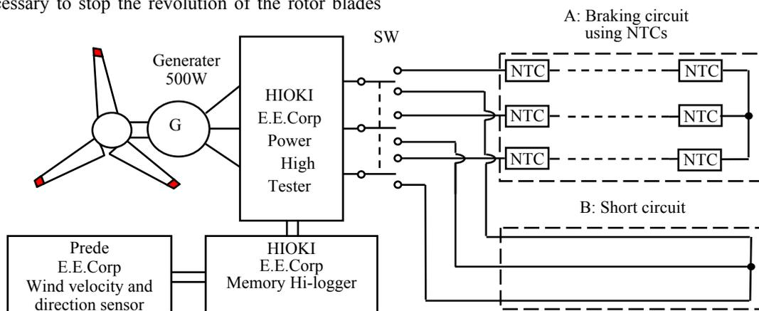
Fig.6. Schematic diagram of experimental device.
