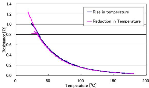
Fig.2. Temperature characteristics of 1R30A
