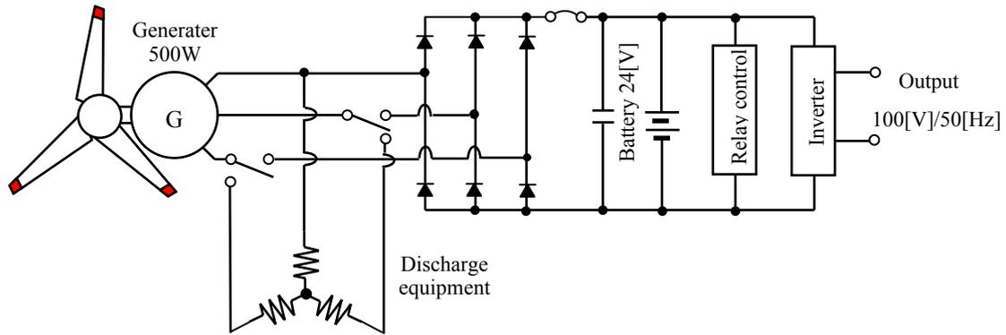
Fig.4. Control system of the small wind turbine.
