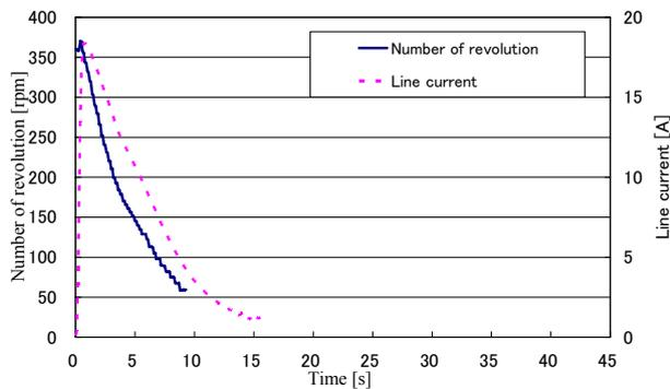
Fig. 8. Number of revolution and line current (short circuit, average wind velocity: 5[m/s]).
